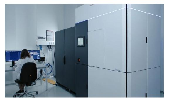
**Galcious 2 Cryo-Transmission Electron Micrscope (cry-TEM)**
